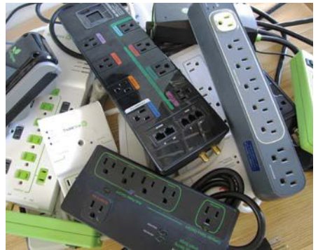
Advanced power strips prevent electronics from drawing energy when they aren't being used.
