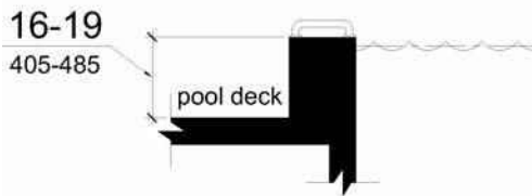
Fig. 75 Transfer Wall Height
