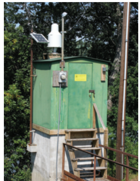
The Middle Atlantic River Forecast Center uses data from USGS stream gages to forecast river stages and flows in the Middle Atlantic Region. USGS field personnel are deployed to stream gage stations during periods of high water to compare stages with flows and help update and improve the Rating Curve.
