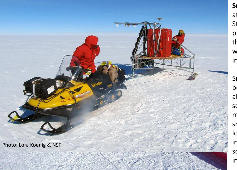
Snow mobiles, here at the South Pole Station with a rugged plastic cargo sled in the foreground and with a passenger sled in the background.
