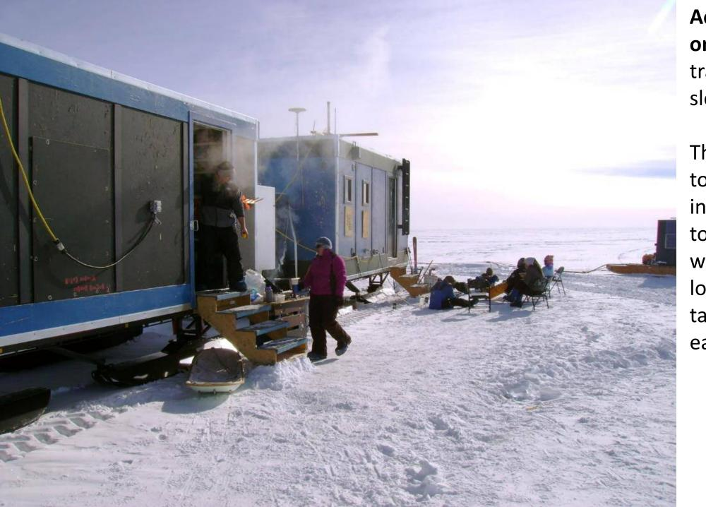
Accommodation units on skis form part of a train of tractor pulled sleds.
