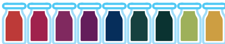
Figure 5. Acid/base (pH color scale): red, pH<3; rose/violet, pH=4-5; blue, pH=6-8; green, pH=9-10; yellow, pH>11.
