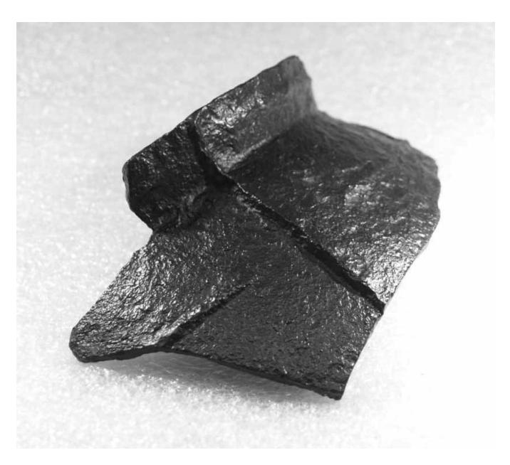
10.11 Fragment (SAIR 2166) showing the misalignment of the two halves of the loam mold. The right side is thicker than the left. The inside of this fragment has no such ridge as the loam core was a single piece with no parting line. (Photograph by Curtis White.)
