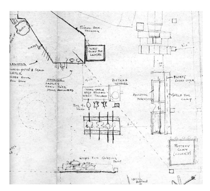
10.8 This drawing proposes how molding operations would be represented in the northeast corner of the casting shed. It includes molding machines, a drying furnace, a bin for mixing loam, and hoops for casting pans (bottom). The circle of dashed lines on the left represents the archeological remains of the casting pit. (Perry, Shaw and Hepburn, Kehoe, and Dean, undated drawing.)
