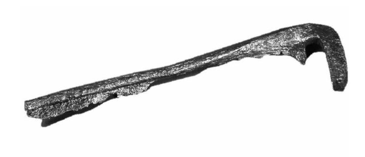
7.4 Scythe blade (SAIR 2585) found at the Joseph Jenks site. In use, a ring held the tang (on the right) of the blade in its wooden handle or snath. A solid mass of iron formed the chine that strengthened the back of the blade. The thin web and edge have rusted away. (Photograph by Curtis White.)
