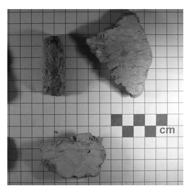
10.13 Pot mold fragments (SAIR 1216) were analyzed by the National Park Service and found to be composed of five parts sand to four parts clay. Drying heat has made the gray clay's outer surfaces a light salmon color. (Photograph by Curtis White.)
