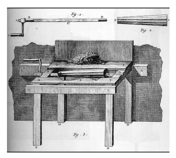
10.12 A loam molding bench with a core-bar, loam, and loam board set in place. Using three such loam boards, the molder and his machine scribed loam into the form of a pot mold. (Plate from Recueil de Planches sur les Sciences, les Arts Liberaux, et les Arts Mechaniques, avec Leur Explication, Troisieme Livraison, Paris, 1765, Forges, 3e Section, Forneau en Merchandise, Moulage en Terre, plate III. Saugus Iron Works NHS.)
