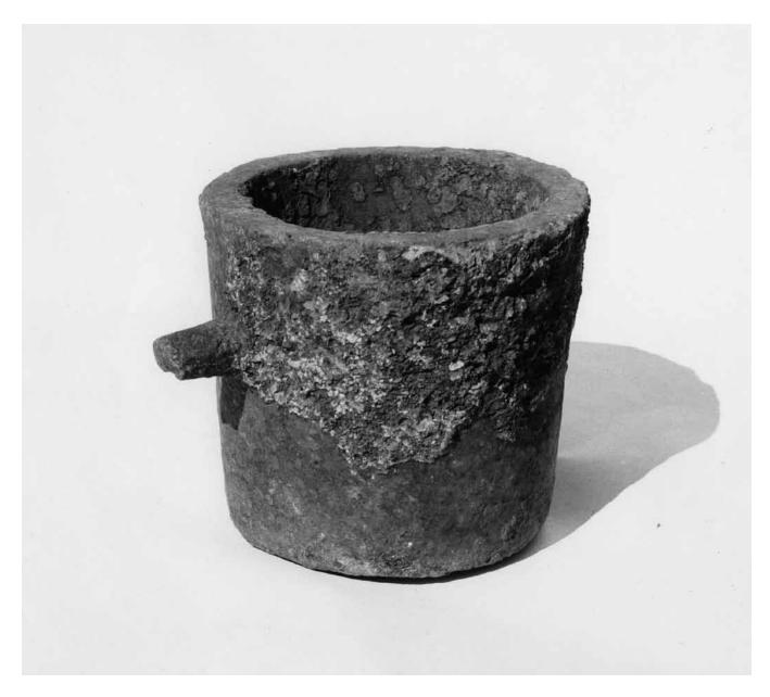
2.9 Saugus crucible used to collect the molten iron from the furnace, which was then ladled out into various molds. (Photograph 1030a by Richard Merrill, 1953.)
