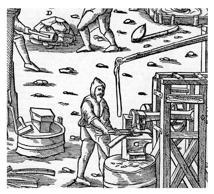
2.11 Detail of water powered hammer similar to the Jenks blacksmith hammer. (Georgius Agricola's 1550 treatise on metallurgy, *De Re Metallica*, p. 422. Courtesy of Dover Publications, Inc. New York, [1950])
