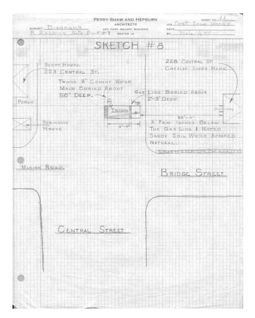
8.9 Robbins' drawing illustrating one of the excavations monitored during utility installation by the town.
