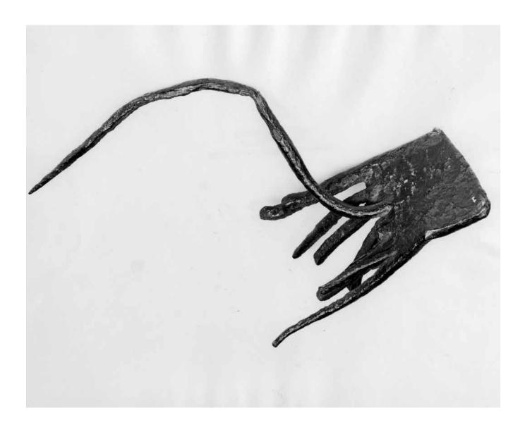
6.17 The partially slit bar (known as the squid) from the slitting mill operation. (Photograph 1180 by Richard Merrill, 1954.)
