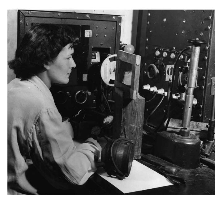
12.18 Technician using spectrometer to examine chemical composition of "Saugus Pot," January 4, 1951. (Photograph 280 by Richard Merrill,1951.)
