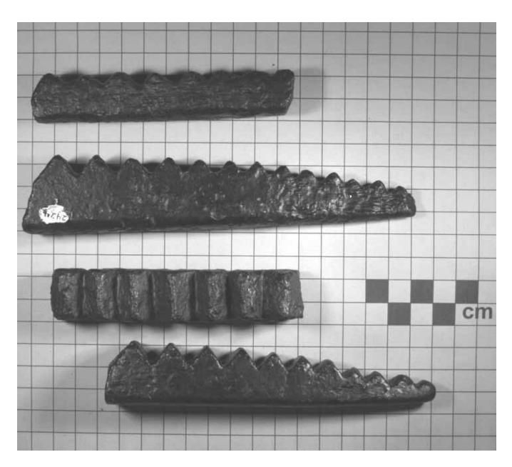
10.9 Four examples of broken "notched bars." First rust and then artifact conservation have rendered the original fracture surfaces indecipherable. (Photograph by Curtis White.)
