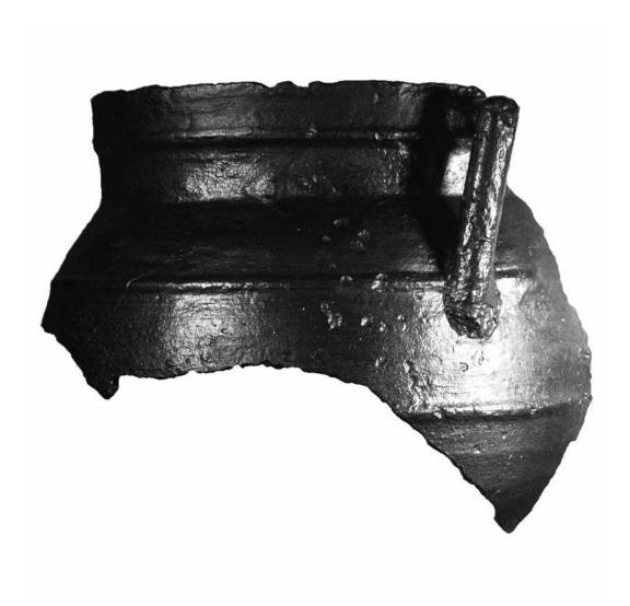
10.10 Typically, cast-iron pots were made from gray cast iron cast in a loam mold. (Photograph by Curtis White.)
