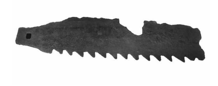
7.5 This broken saw blade was made for a saw mill and found in ruins of the Jenks shop. An iron rod would have passed through the square hole to attach the blade to a sash that reciprocated with the help of a pitman arm attached to the waterwheel. Saw blades such as these could be ganged together to make multiple cuts with a single pass through the mill (Photograph by Dan Boivin.)
