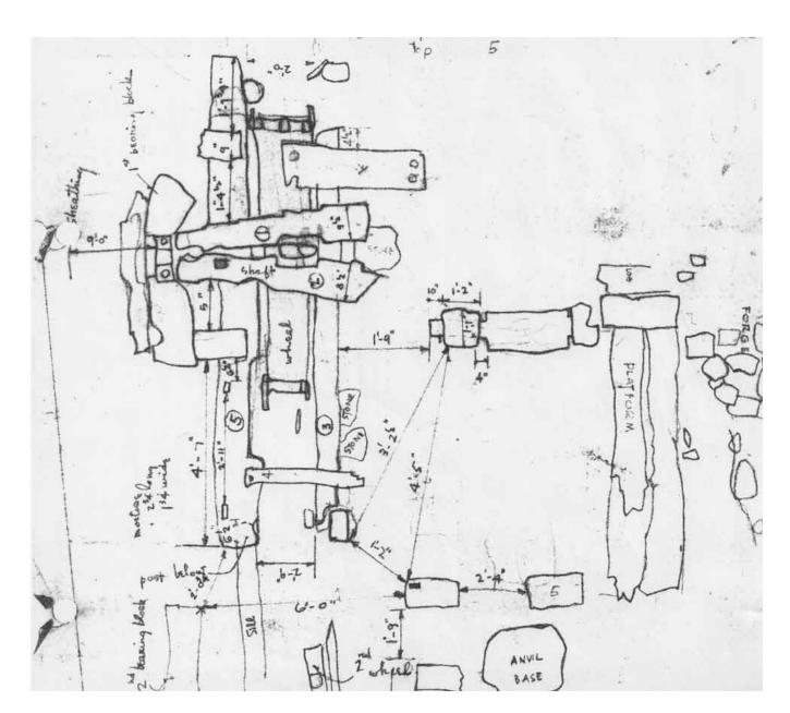
7.11 Detail of drawing of Jenks' hammer assembly including: an overshot waterwheel and shaft, hutch, bearing block, fulcrum (as Robbins called it)and anvil base. Forge and floorboards can be seen on the right. (Perry, Shaw and Hepburn, Kehoe and Dean drawing, March 26, 1952.)
