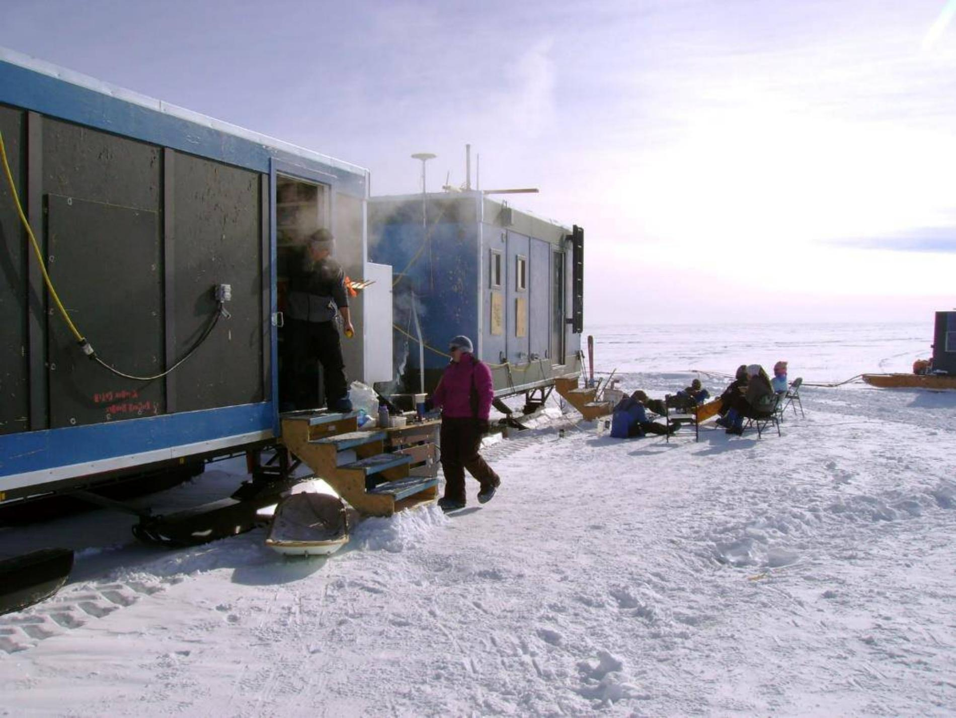
**Accommodation units on skis** form part of a train of tractor pulled sleds.
