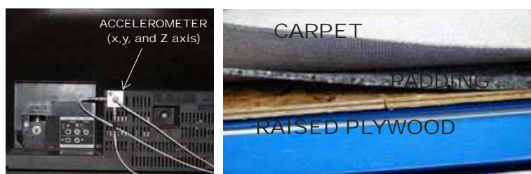
Figure 3. Accelerometer and flooring test set-up
